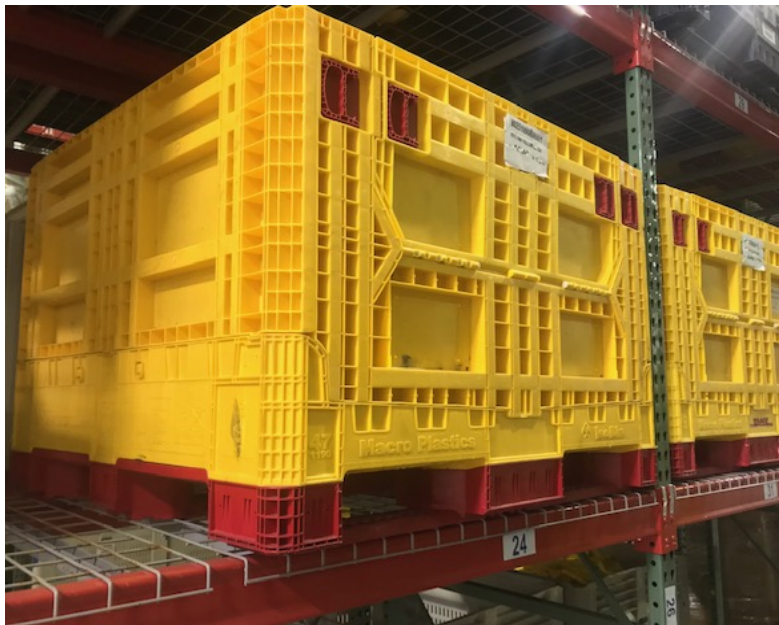
Bins safely stacked on fully supported deck racking Bins must NEVER be beam or edge racked
