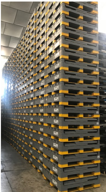
Bins safely stacked on level floor
